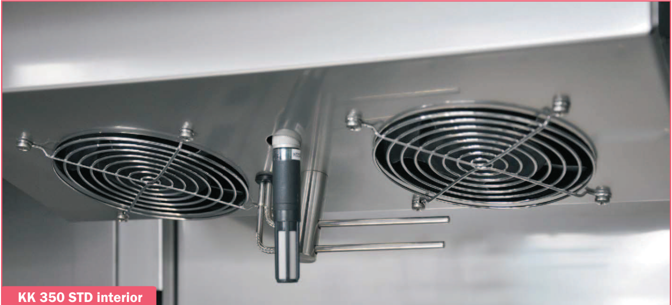
Temperature and humidity sensors in the interior of a climatic chamber.
