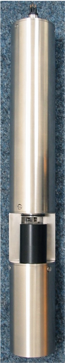
Fig. 3 ProPS (ClearWater) with a adapter tube for 10mm optical pathlength in water
